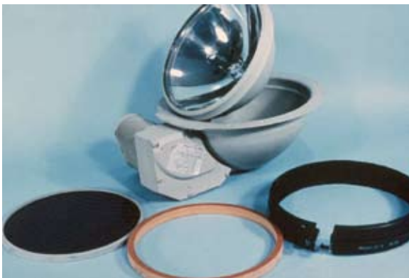
C-130 Landing Light and Blacked-Out Lighting Modification Parts.
