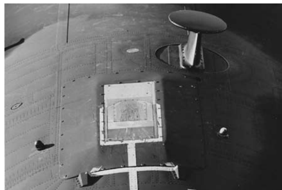
SATCOM Hatch-Mounted Antenna in Proximity to C-130 Airborne Refueling Receptacle
