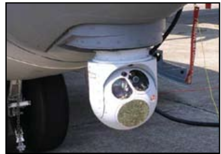
The MC-130W’s nose houses a AN/APN-241 Low Power Color weather/navigation Radar and a AN/AAQ-38 forward looking infrared (FLIR) pod in a chin turret.
